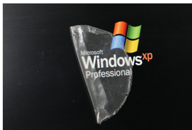
Figure 4. An ionically modified flexible and transparent BIMS film (B-40). [Color figure can be viewed in the online issue, which is available at wileyonlinelibrary.com .]
